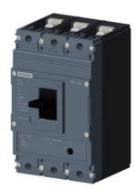
circuit breaker 3VJ1 IEC framesize 3VJ11 125A line protection ATFM 3-pole Icu=25kA@415V Ics=75% Icu In=125A overload protection Ir=100A...125A shortcircuit protection Ii=10 x In Screw connection
