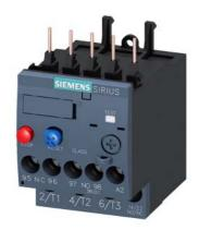
Overload relay 0.70...1.0 A Thermal For motor protection Size S00, Class 10 Contactor mounting Main circuit: Screw Auxiliary circuit: Screw Manual-Automatic-Reset
