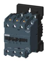
3P Power Contactor AC3:40A 1NO+1NC AC220V 50/60Hz Main circuit: Screw Auxiliary circuit: Screw
