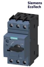
Circuit breaker size S0 for motor protection, CLASS 10 A-release 18...25 A N-release 325 A Screw terminal Standard switching capacity
