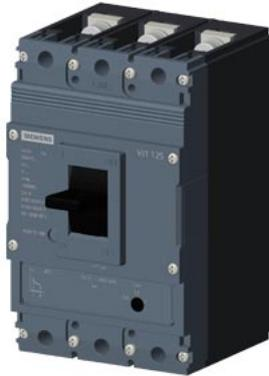
circuit breaker 3VJ1 IEC framesize 3VJ11 125A line protection ATFM 3-pole Icu=25kA@415V Ics=75% Icu In=100A overload protection Ir=80A...100A short-circuit protection li=10 x In Screw connection
