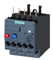
Overload relay 0.14...0.20 A Thermal For motor protection Size S00, Class 10 Contactor mounting Main circuit: Screw Auxiliary circuit: Screw Manual-Automatic-Reset
