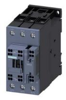
power contactor, AC-3e/AC-3, 65 A, 30 kW / 400 V, 3-pole, 110 V AC, 50/60 Hz, auxiliary contacts: 1 NO + 1 NC, main circuit: screw terminal, control and auxiliary circuit: spring-loaded terminal, size: S2
