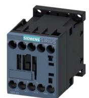
power contactor, AC-3e/AC-3, 12 A, 5.5 kW / 400 V, 3-pole, 110 V AC, 50/60 Hz, auxiliary contacts: 1 NO, screw terminal, size: S00
