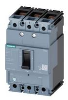
circuit breaker 3VM1 IEC frame 160 breaking capacity class N Icu=25kA @ 415V 3-pole, line protection TM220, ATFM, In=50A overload protection Ir=35A...50A short-circuit protection Ii=10 x In nut keeper kit
