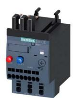
Overload relay 2.8...4.0 A Thermal For motor protection Size S00, Class 10 Contactor mounting Main circuit: Spring-type terminal Auxiliary circuit: spring-type terminal Manual-Automatic-Reset
