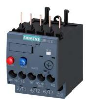
Overload relay 0.11...0.16 A Thermal For motor protection Size S00, Class 10 Contactor mounting Main circuit: Screw Auxiliary circuit: Screw Manual-Automatic-Reset
