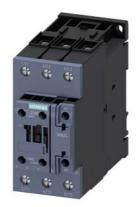
power contactor, AC-3e/AC-3, 41 A, 18.5 kW / 400 V, 3-pole, 220 V AC, 50/60 Hz, auxiliary contacts: 1 NO + 1 NC, screw terminal, size: S2
