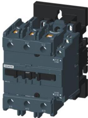
3P Power Contactor AC3:80A 1NO+1NC AC220V 50/60Hz Main circuit: Screw
