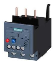
Overload relay 28...40 A Thermal For motor protection Size S2, Class 10 Contactor mounting Main circuit: Screw Auxiliary circuit: Screw Manual-Automatic-Reset
