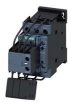
capacitor contactor, AC-6b 25 kVAr, / 400 V, 3-pole, 230 V AC, 50/60 Hz, auxiliary contacts: 1 NO + 2 NC, screw terminal, size: S0
