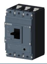
circuit breaker 3VJ1 IEC framesize 3VJ11 125A line protection ATFM 3-pole Icu=25kA@415V Ics=75% Icu In=50A overload protection Ir=40A...50A short-circuit protection Ii=600A Screw connection
