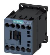
power contactor, AC-3e/AC-3, 12 A, 5.5 kW / 400 V, 3-pole, 220 V AC, 50/60 Hz, auxiliary contacts: 1 NC, screw terminal, size: S00
