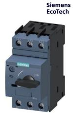
Circuit breaker size S0 for motor protection, CLASS 10 A-release 3.5...5 A N release 65 A screw terminal Standard switching capacity
