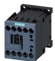
power contactor, AC-3e/AC-3, 7 A, 3 kW / 400 V, 3-pole, 24 V DC, auxiliary contacts: 1 NC, screw terminal, size: S00
