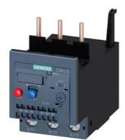
Overload relay 62...73 A Thermal For motor protection Size S2, Class 10A Contactor mounting Main circuit: Screw Auxiliary circuit: spring-type terminal Manual-Automatic-Reset
