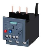
Overload relay 14...20 A Thermal For motor protection Size S2, Class 10 Contactor mounting Main circuit: Screw Auxiliary circuit: Screw Manual-Automatic-Reset
