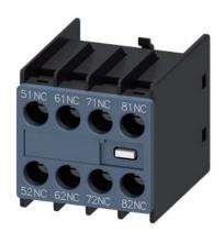
auxiliary switch, on the front, 4 NC, 51/52, 61/62, 71/72, 81/82, current path: 1 NC, 1 NC, 1 NC, 1 NC, screw terminal, physically coded, only with contactor relays 3RH2140 and 3RH2440 combinable (according to EN 50011)
